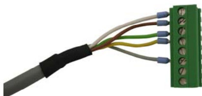
Figure 4. Connector wiring GXR-GPS
