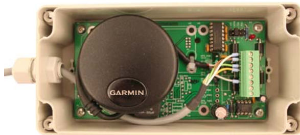
Figure 12. Inside view of the GXR-GPS housing
