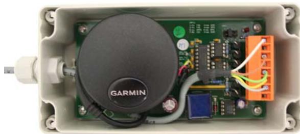
Figure 13. Inside view of the GXR-GPS-485 housing
