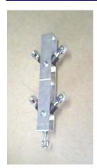
tubing, generally installed within installation time. drilled hole, used conjunction with a wheeled sensor probe system to determine sub-surface ground dynamic movements. internal grooves provide an orientation reference for the inclinometer probe readings. attention is paid to minimise the twisting of the casing grooves.
