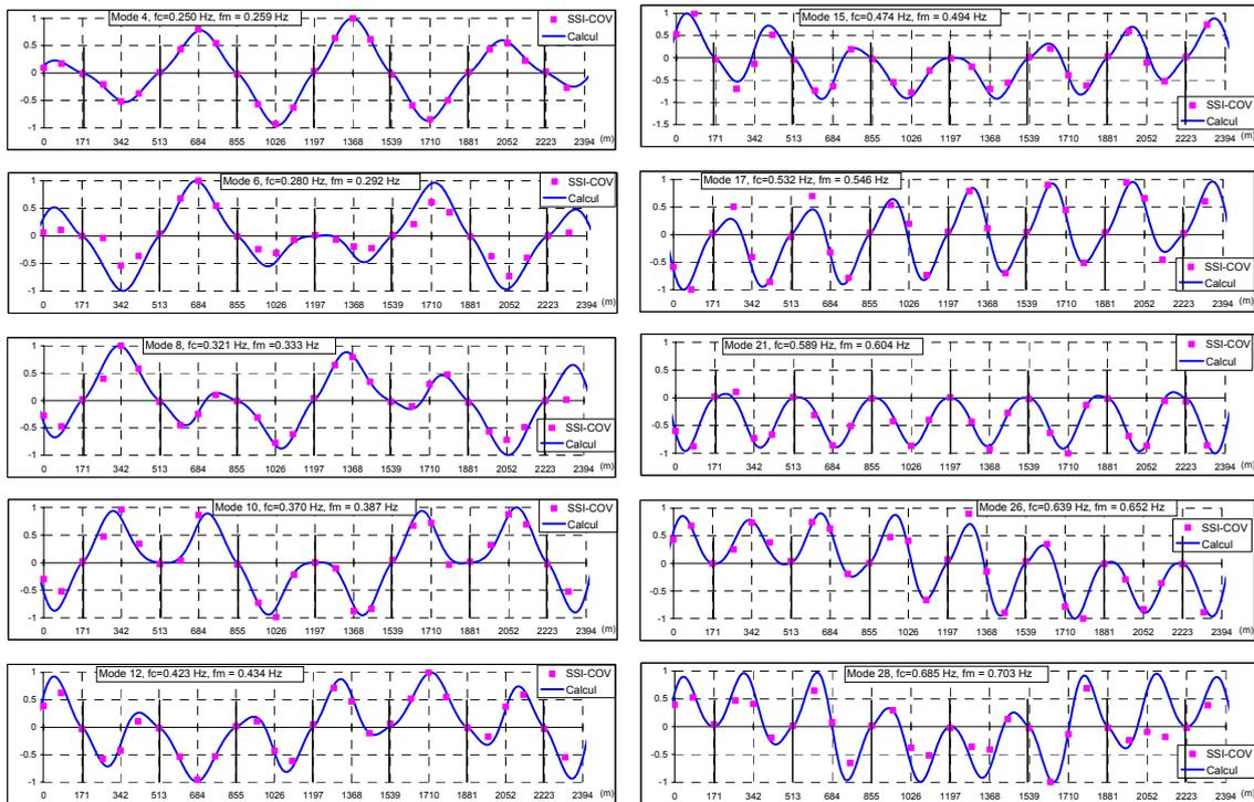
Figure 15. Vertical bending modes in the range 0.2-0.7Hz: identified vs calculated modal components
