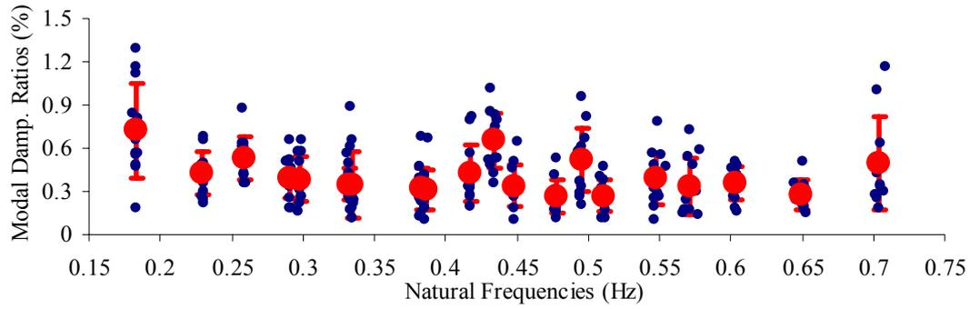
Figure 8. Identified natural frequencies and modal damping ratios: values estimated in each setup and final results represented by the average values and by an interval of variation for the modal damping ratios based on the standard deviation (average  $\pm$  standard deviation).
