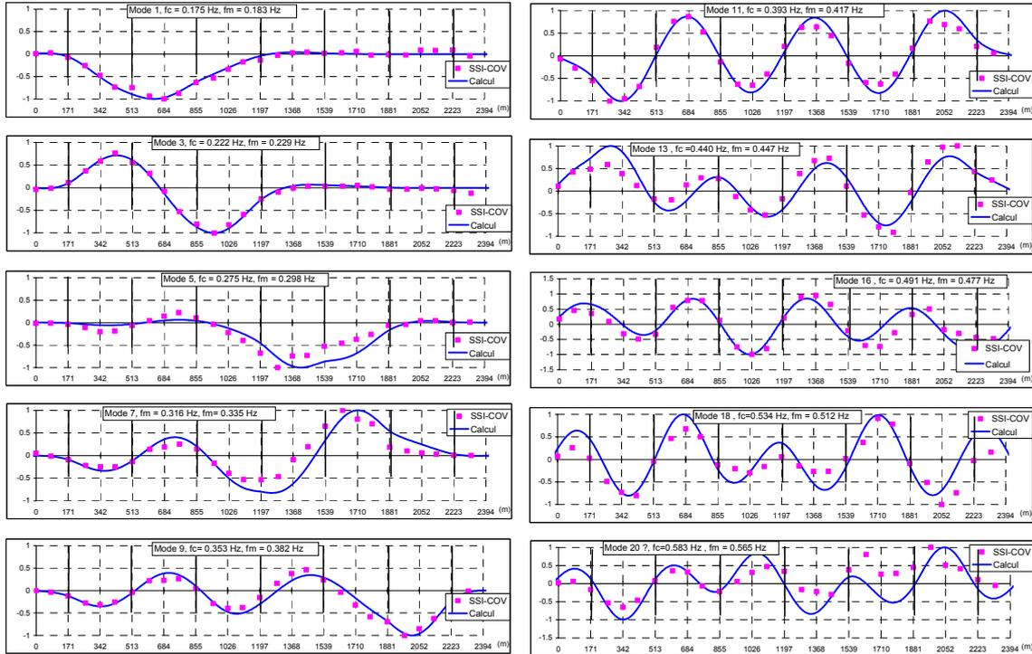
Figure 16. Transversal bending modes in the range 0.1-0.6Hz: identified vs calculated modal components
