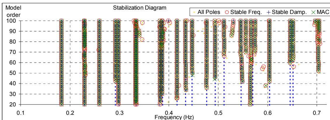
Figure 11. Stabilization diagram of the single analysis – SSI-COV
