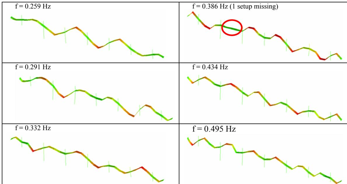
Figure 9. First six vertical identified mode shapes
