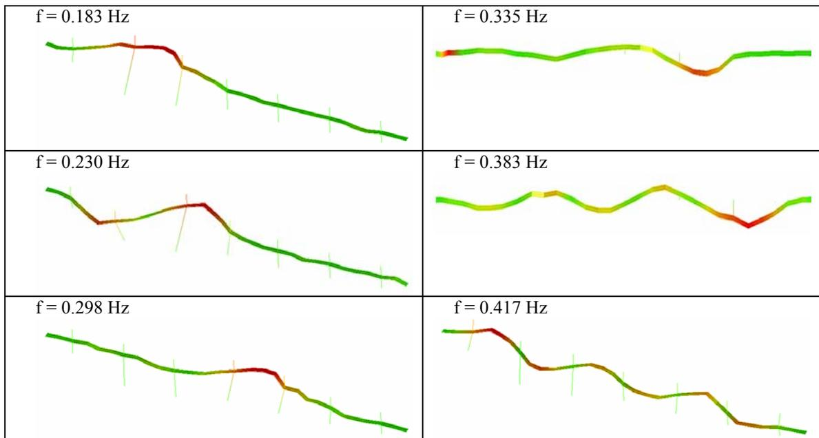
Figure 10. First six lateral identified mode shapes
