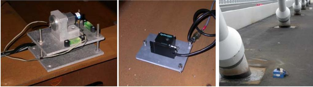
Figure 3. Accelerometers installed inside the deck and seismograph used outside
