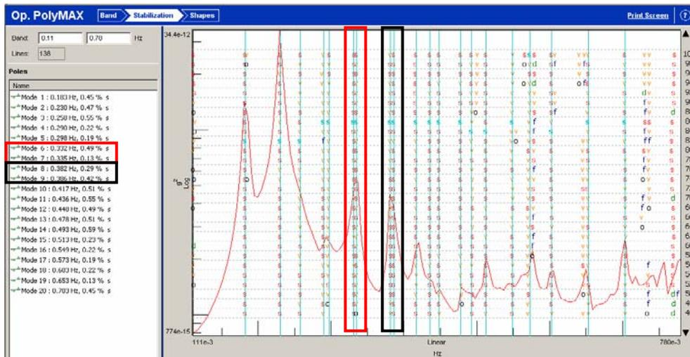
Figure 7. Stabilization diagram of the 4<sup>th</sup> setup - PolyMax method
