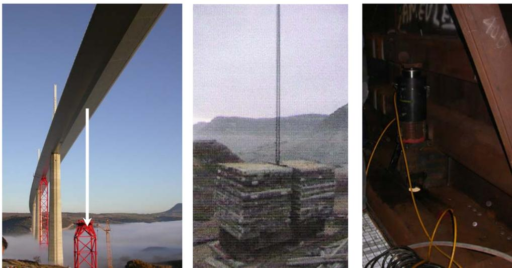
Figure 5. Free vibration test: tensioned cable, cut from inside the box girder
