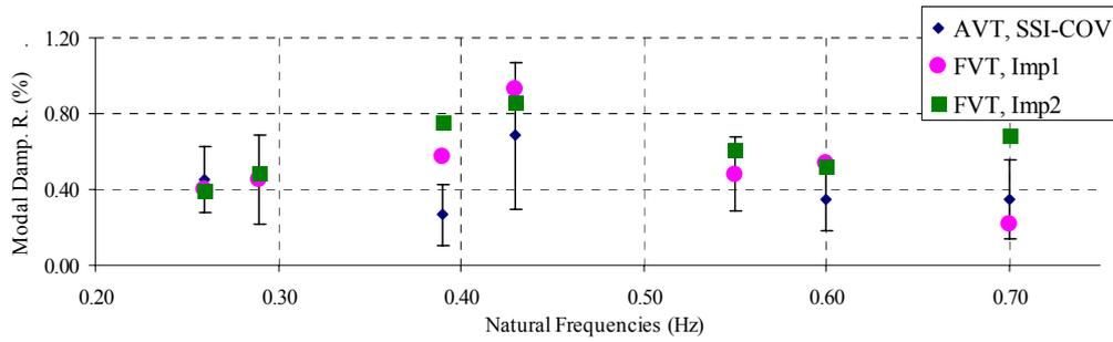
Figure 14. Modal damping ratios obtained from the Ambient Vibration Test (AVT) and from the Free Vibration tests (FVT). Imp1 – 600kNmass; Imp2 – 1000kN mass.
