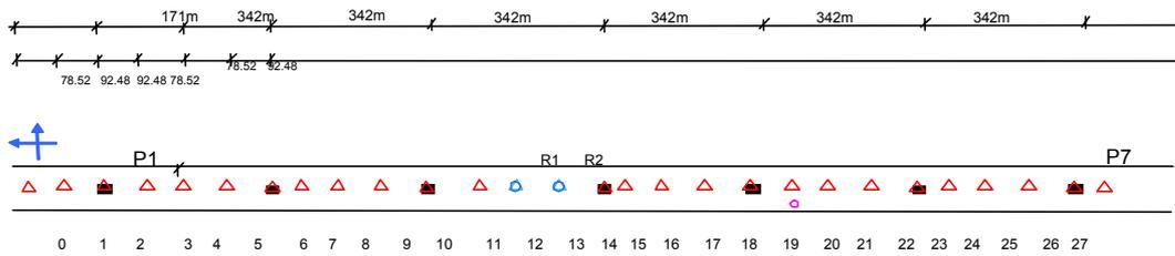
Figure 4. Instrumented sections of the deck in the ambient vibration test
