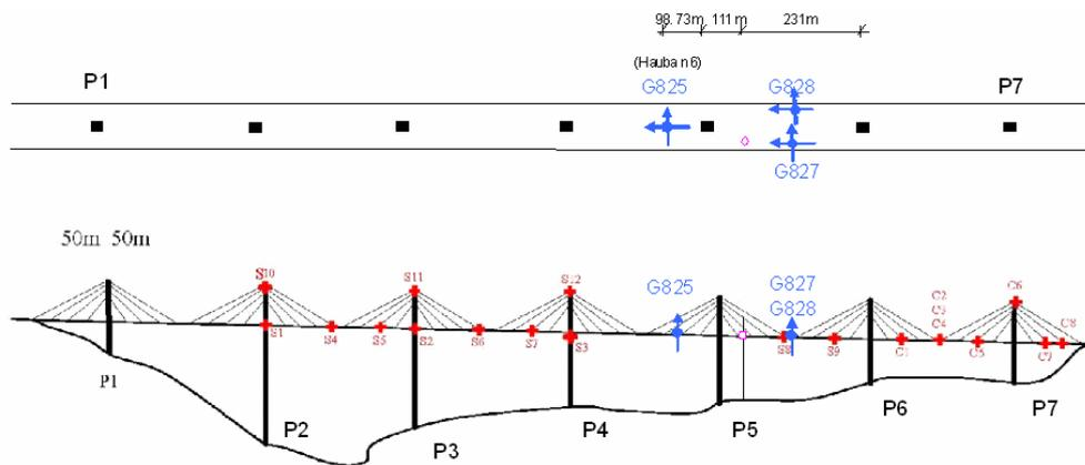
Figure 2. Location of the instrumentation used in the free vibration test
