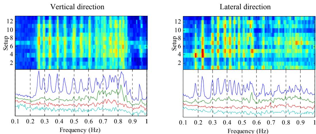
Figure 6. Average singular values of the spectra matrices and colour maps with the variation of the 1<sup>st</sup> singular values during the ambient vibration test.
