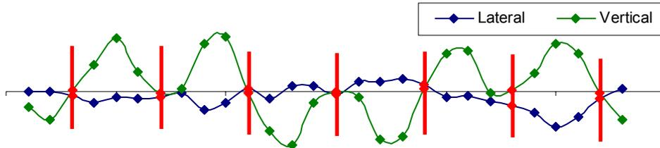
Figure 12. 4<sup>th</sup> vertical mode shape ( $f = 0.386\text{Hz}$ ), not well identified with the multiple analyses
