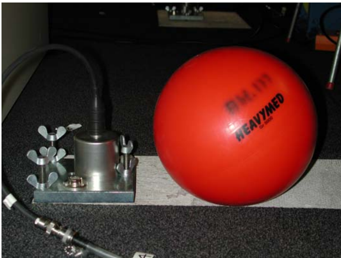
Figure 4: The medical ball used to excite the slabs and one of the accelerometers used to measure the slab response.
