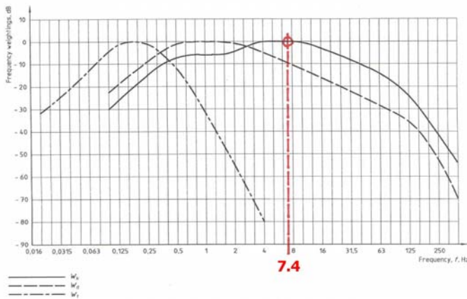
Figure 17. Frequency weighting curves as given in ISO 2631-1 (1997). W_k (solid line) applies for vertical movement.
